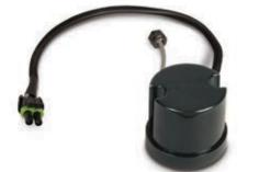
The P2.0 Position Control is a microprocessor position feedback control providing a 0-10 volt DC output indicating actuator travel. The control uses two inductive pulse count sensors and a counting wheel to accurately determine actuator position. A third sensor at the full retract position provides a zero or home position indication.
